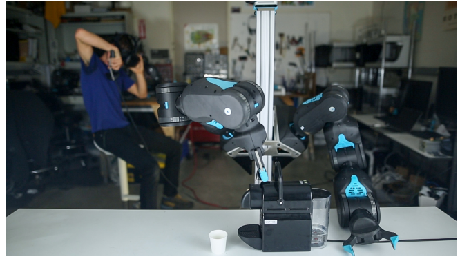
Fig. 5. Blue completely teleoperates an espresso machine. A Virtual Reality operator (in background) pilots Blue using an HTC Vive system through a Unity bridge. A predictable 7-DoF ‘elbows out’ configuration is interpreted from 6-DoF Vive controller pose. Visual feedback is provided by an Intel RealSense D415 depth camera. [video on website]
