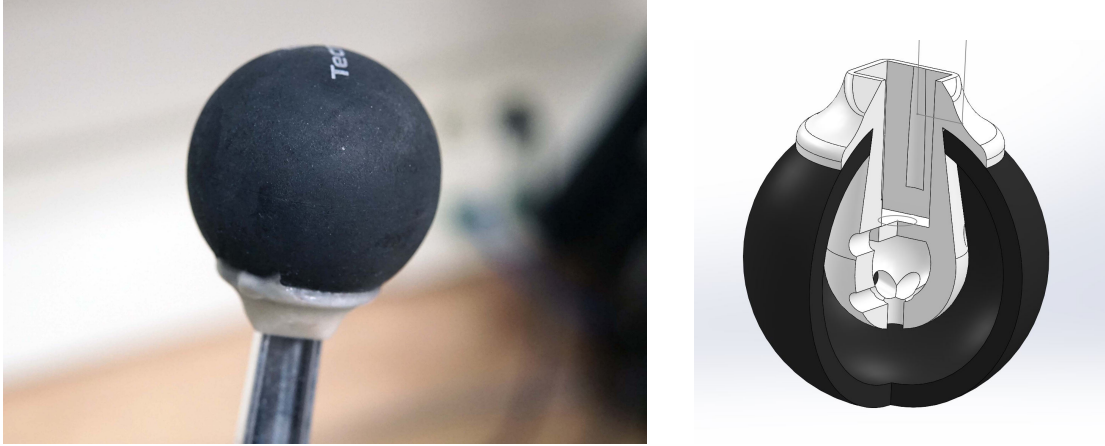
Figure 3-12: Foot, and cross section(Left). The plastic insert has holes which are filled by the casting foam.
