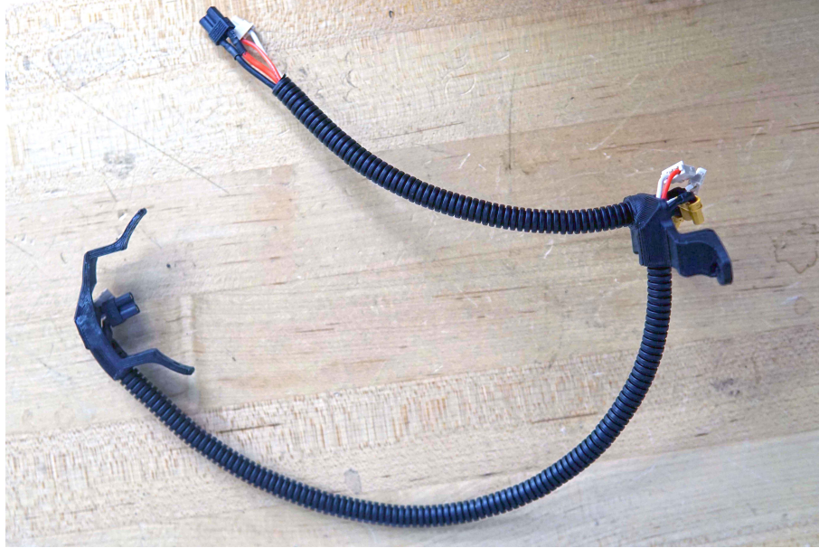
Figure 3-13: Wiring harness for one leg. Flexible wires are housed within protective corrugated sheaths, which are fixed by 3D printed guides at each end, strain-relieving the connectors.
