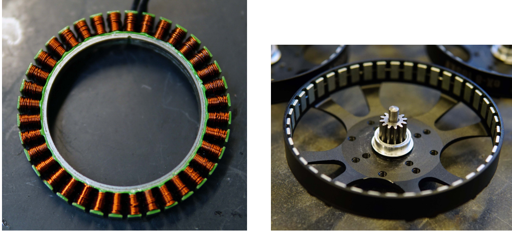
Figure 2-4: Stator (left) and rotor (right) of the brushless motor used in the actuator. The rotor has been modified to fit the sun gear of the planetary transmission.
