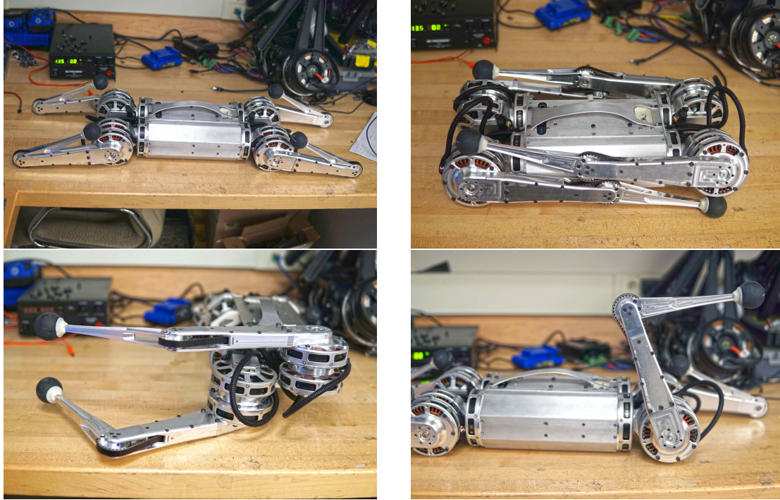
Figure 3-3: A variety of configurations possible with the wide range of motion of the legs. Top Left: Turn-on configuration. In this configuration the legs are correctly zeroed for turn-on. Top Right: The robot can be folded up for transportation. Bottom Left: The ab/ad joints have enough range of motion for the robot to walk with the body rolled \pm 90^\circ . Bottom Right: The legs can be lifted above the body, for climbing very tall obstacles or manipulation.
