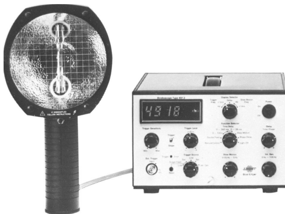
FIGURE 10.16 A stroboscope. (Courtesy of Bruel and Kjaer Instruments, Inc., Marlborough, MA.)
