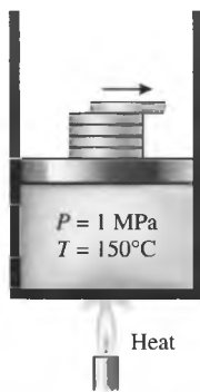
FIGURE 3-19 The pressure in a piston-cylinder device can be reduced by reducing the weight of the piston.
