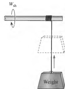
FIGURE 7-23 In the absence of friction, raising a weight by a rotating shaft does not create any disorder (entropy), and thus energy is not degraded during this process.
