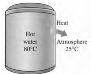
FIGURE 8-18 The second-law efficiency of naturally occurring processes is zero if none of the work potential is recovered.
