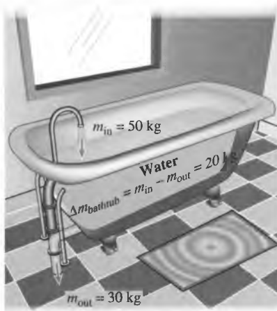
FIGURE 5-5 Conservation of mass principle for an ordinary bathtub.
