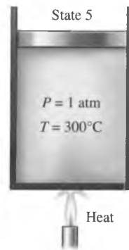
FIGURE 3-10 As more heat is transferred, the temperature of the vapor starts to rise ( superheated vapor ).
