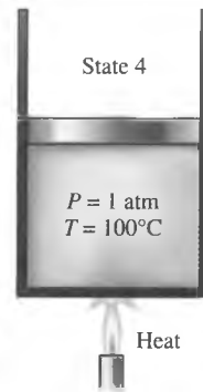
FIGURE 3-9 At 1 atm pressure, the temperature remains constant at 100^\circ\text{C} until the last drop of liquid is vaporized ( saturated vapor ).
