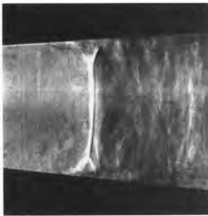
FIGURE 17-30 Schlieren image of a normal shock in a Laval nozzle. The Mach number in the nozzle just upstream (to the left) of the shock wave is about 1.3. Boundary layers distort the shape of the normal shock near the walls and lead to flow separation beneath the shock.
