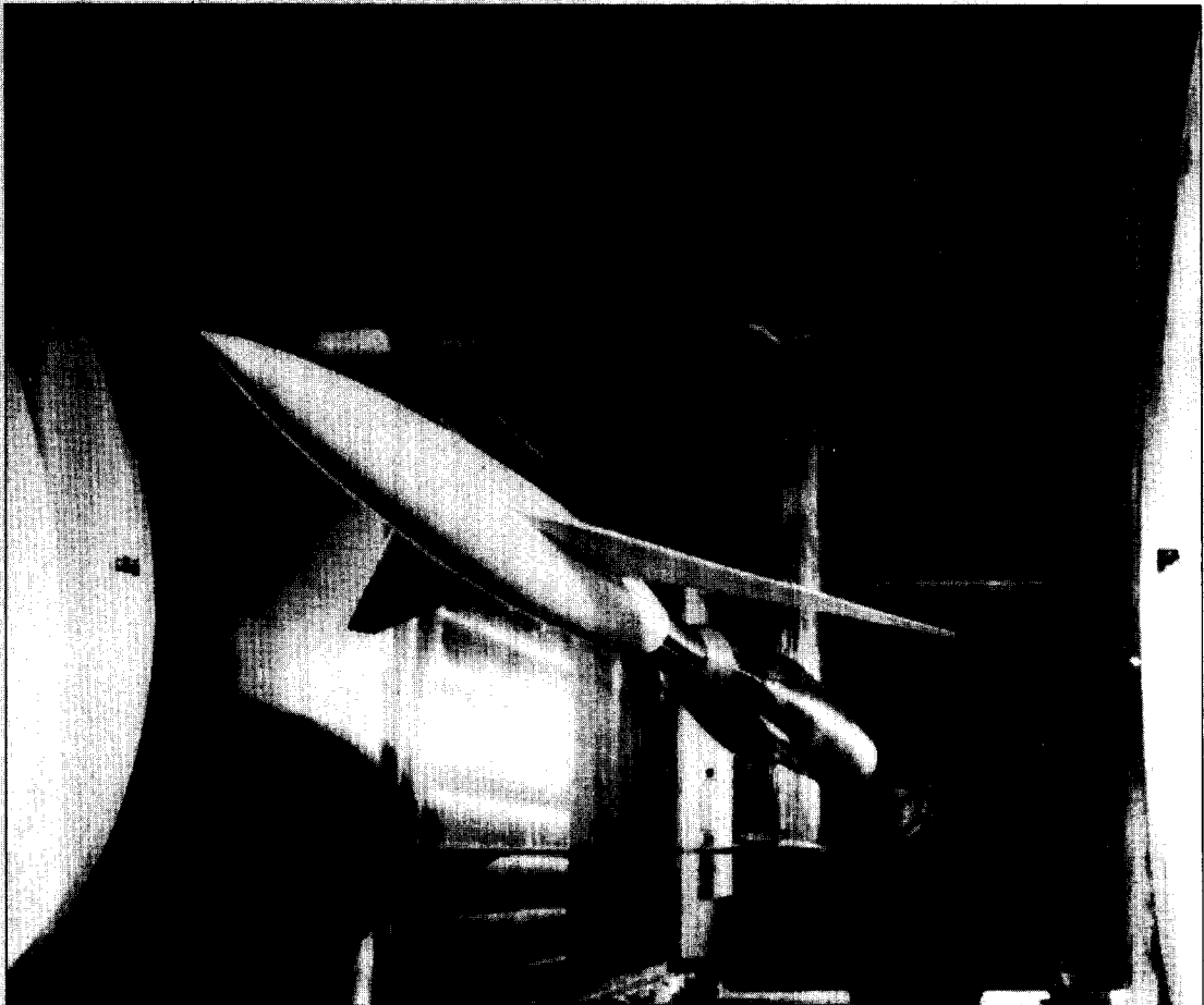
Figure 5.2 | An aircraft model mounted in the test section of the Ames 6 × 6-foot supersonic wind tunnel. The test section is labeled as item 2 in Fig. 5.1.
