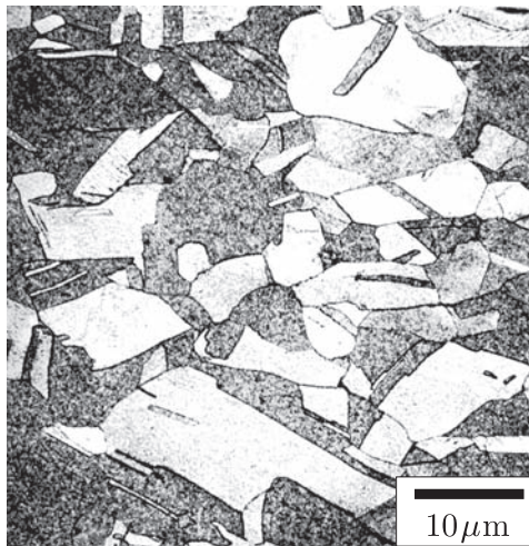
Figure 102.1. Photomicrograph of a metal. At the microstructural scale most metals are an aggregate of a large number of single crystals. The single crystals are called grains, and these are separated by grain boundaries.
