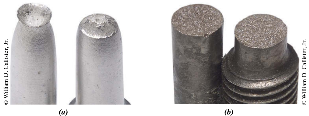
Figure 9.3 (a) Cup-and-cone fracture in aluminum. (b) Brittle fracture in a gray cast iron.
