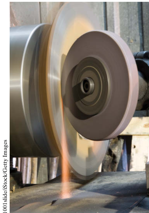
Figure 13.13 Photograph of a clutch lining pressure plate that is being ground with a grinding wheel.
