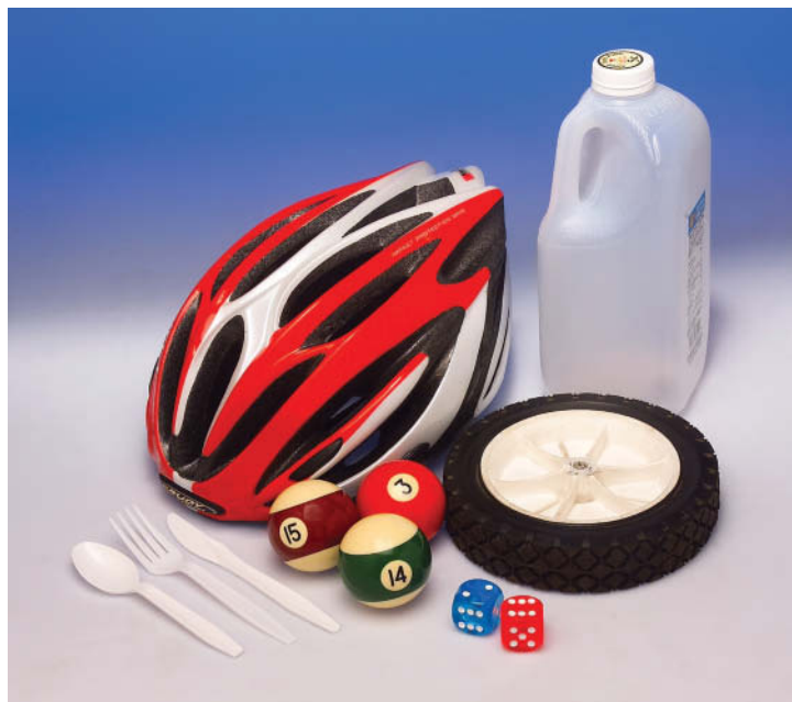
Figure 1.11 Several common objects made of polymeric materials: plastic tableware (spoon, fork, and knife), billiard balls, a bicycle helmet, two dice, a lawn mower wheel (plastic hub and rubber tire), and a plastic milk carton.
