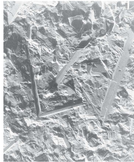
Figure 13.10 Scanning electron micrograph showing the microstructure of a glass-ceramic material. The long, acicular, blade-shaped particles yield a material with unusual strength and toughness. 37,000 \times . (Photograph courtesy of L. R. Pinckney and G. J. Fine, Corning Incorporated.)
