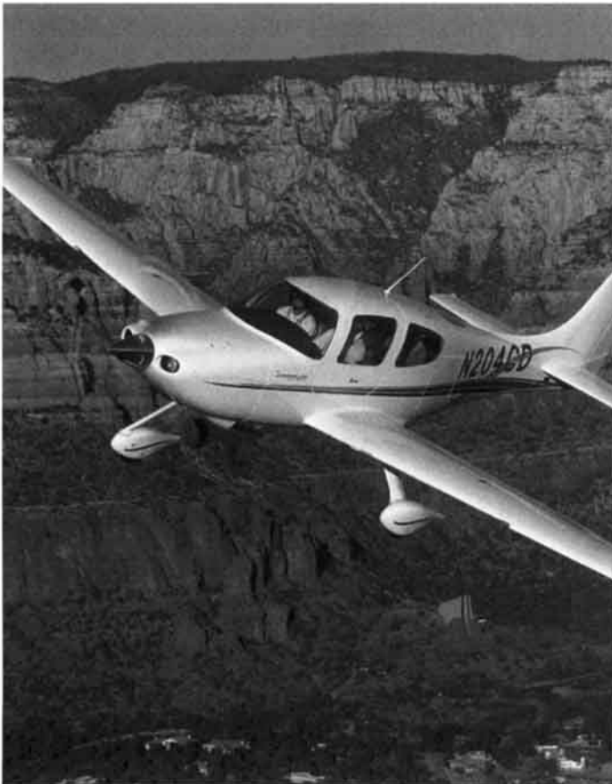
Fig. 1.6 Small aircraft with primary structure made of composite materials. (Courtesy of Dr. Paul Brey, Cirrus Design Corporation.)
