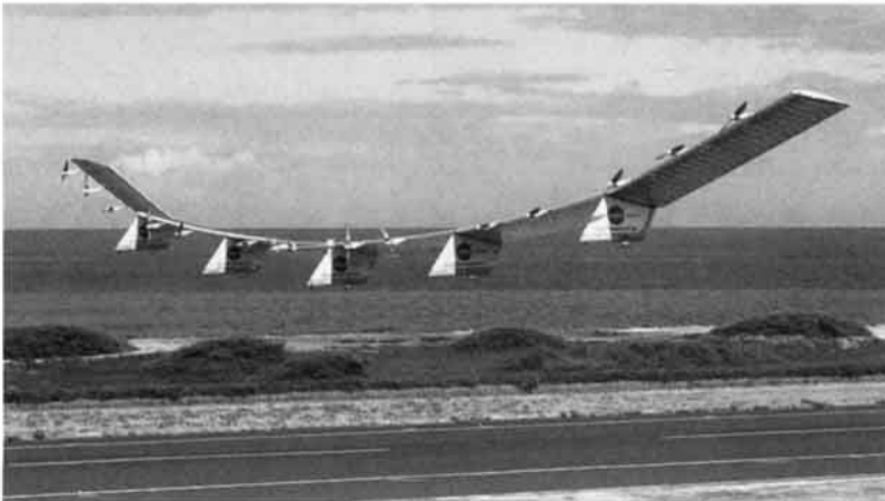
Fig. 1.9 Solar-powered flying wing Helios. (Courtesy of Stuart Hindle, Sky Tower, Inc.; NASA Dryden Flight Center photograph.) 3
