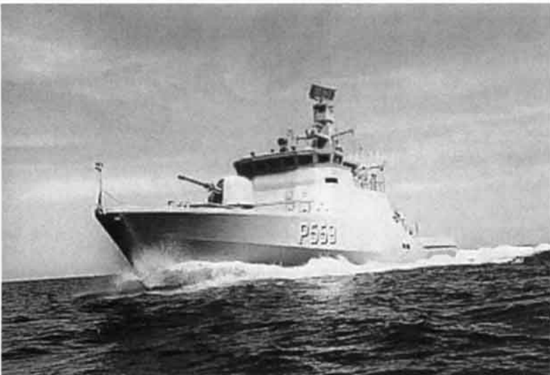
Fig. 1.12 Royal Danish Navy standard Flex 300 corvette: length, 55 m; displacement, 350 tons; materials, glass/polyester and PVC foam. (Courtesy of Professor Ole Thomsen, Aalborg University, Denmark.)
