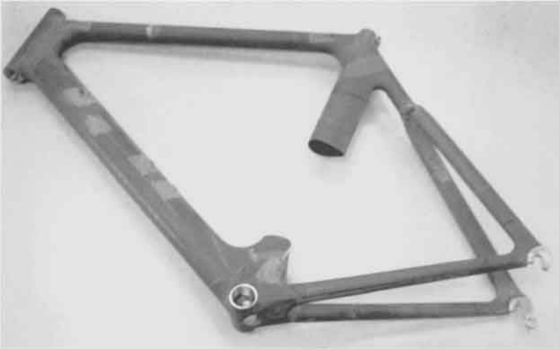
Fig. 1.18 Bicycle frame made of carbon/epoxy composite and weighing 1.36 kg (3 lb), which is much less than the 5 kg (11 lb) weight of the corresponding steel frame.
