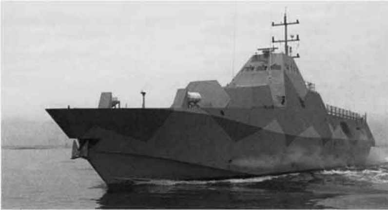
Fig. 1.13 Royal Swedish Navy Visby class corvette: length, 72 m; displacement, 600 tons; materials, carbon/vinylester and PVC foam. (Courtesy of Professor Christian Berggreen, Technical University of Denmark and Kockums AB, Malmö, Sweden.)
