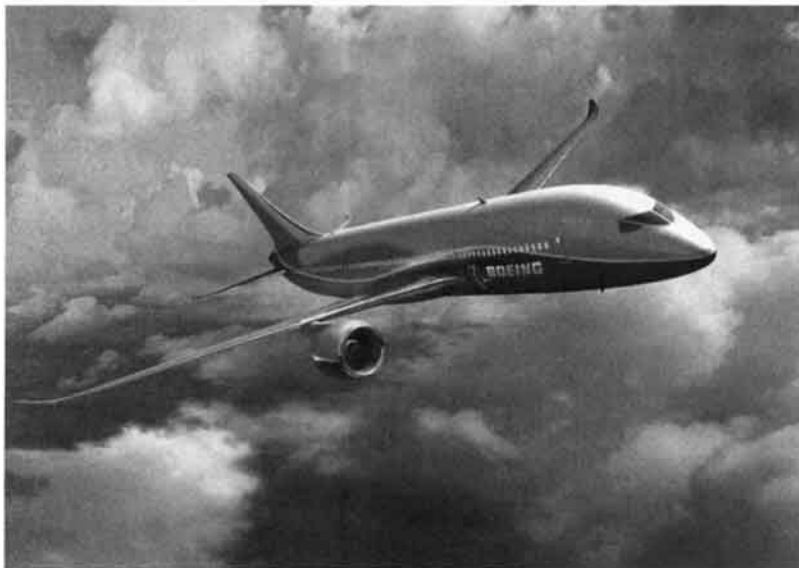
Fig. 1.4 Boeing 787 “Dreamliner” with most of the fuselage and wings made of composite materials. (Courtesy Boeing Commercial Airplane Group.)
