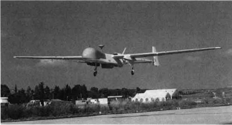
Fig. 1.8 Unmanned reconnaissance aircraft made of composite materials. (Courtesy of MALAT Division, Israel Aircraft Industries.)
