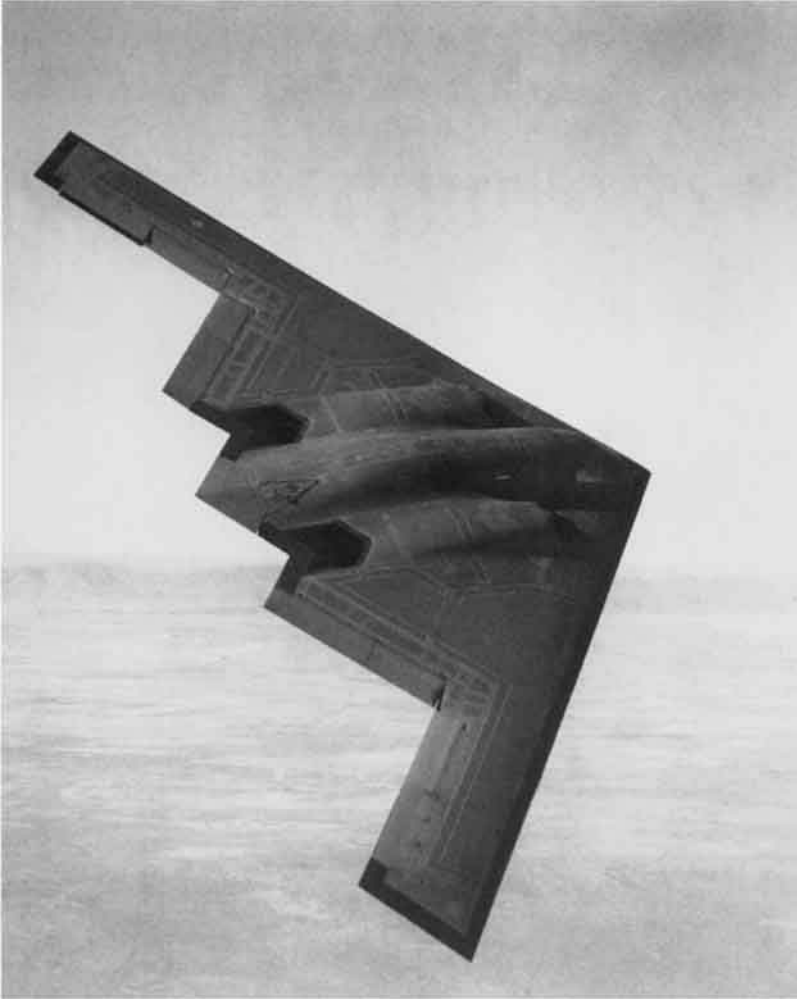
Fig. 1.7 B-2 stealth bomber made almost entirely of composite materials. (Courtesy of Dr. R. Ghetzler, Northrop Corporation.)
