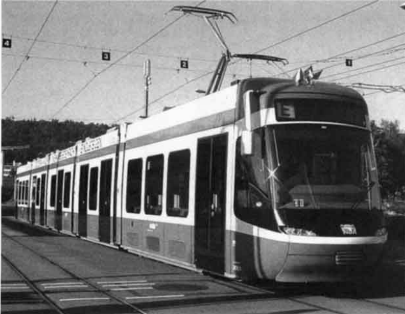
Fig. 1.11 Cobra tram in Zurich, Switzerland, incorporating composite sandwich construction. (Courtesy of Alcan Airex AG, photograph by Bombardier Transportation.)
