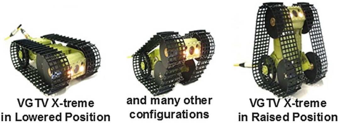
Disaster Response Robot, Fig. 3 VGTV X-treme (Courtesy of Recce Robotics) http://www.recce-robotics.com/vgtv.html
