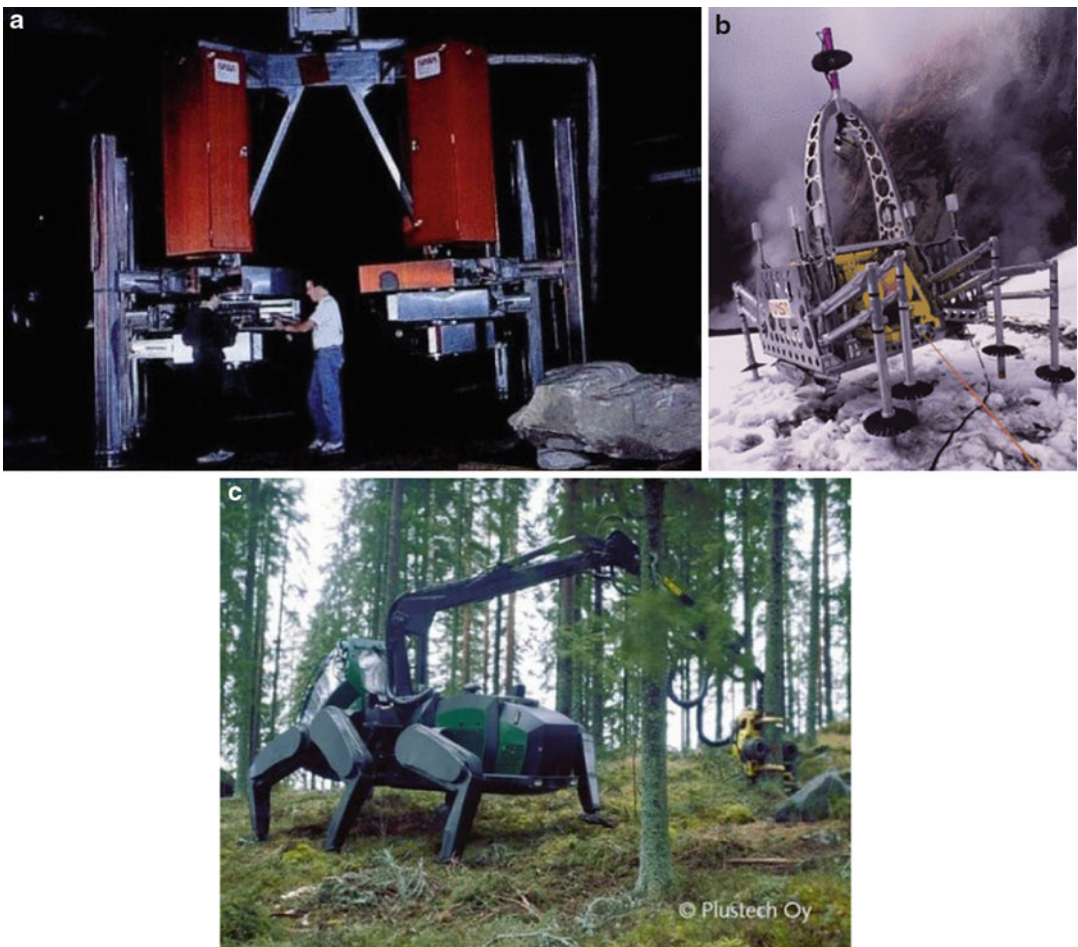
Walking Robots, Fig. 6 Large walking robots: (a) Dante II, CMU; (b) Ambler, CMU; and (c) John Deere Walking Tractor
