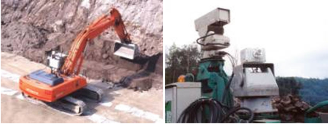
Disaster Response Robot, Fig. 2 Unmanned construction system (Courtesy of Society for Unmanned Construction Systems) http://www.kenmukyou.gr.jp/f_souti.htm
