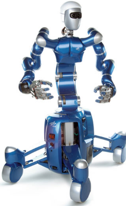
Redundant Robots, Fig. 6 The DLR rolling justin
