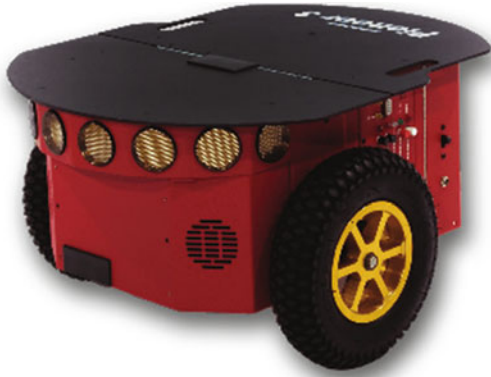
Wheeled Robots, Fig. 1 The Pioneer by Adept is a popular differential-drive platform
