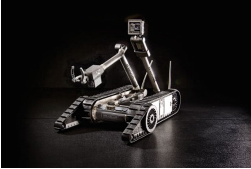
Disaster Response Robot, Fig. 6 PackBot (Courtesy of iRobot) http://www.irobot.com/us/learn/defense/packbot/Specifications.aspx
