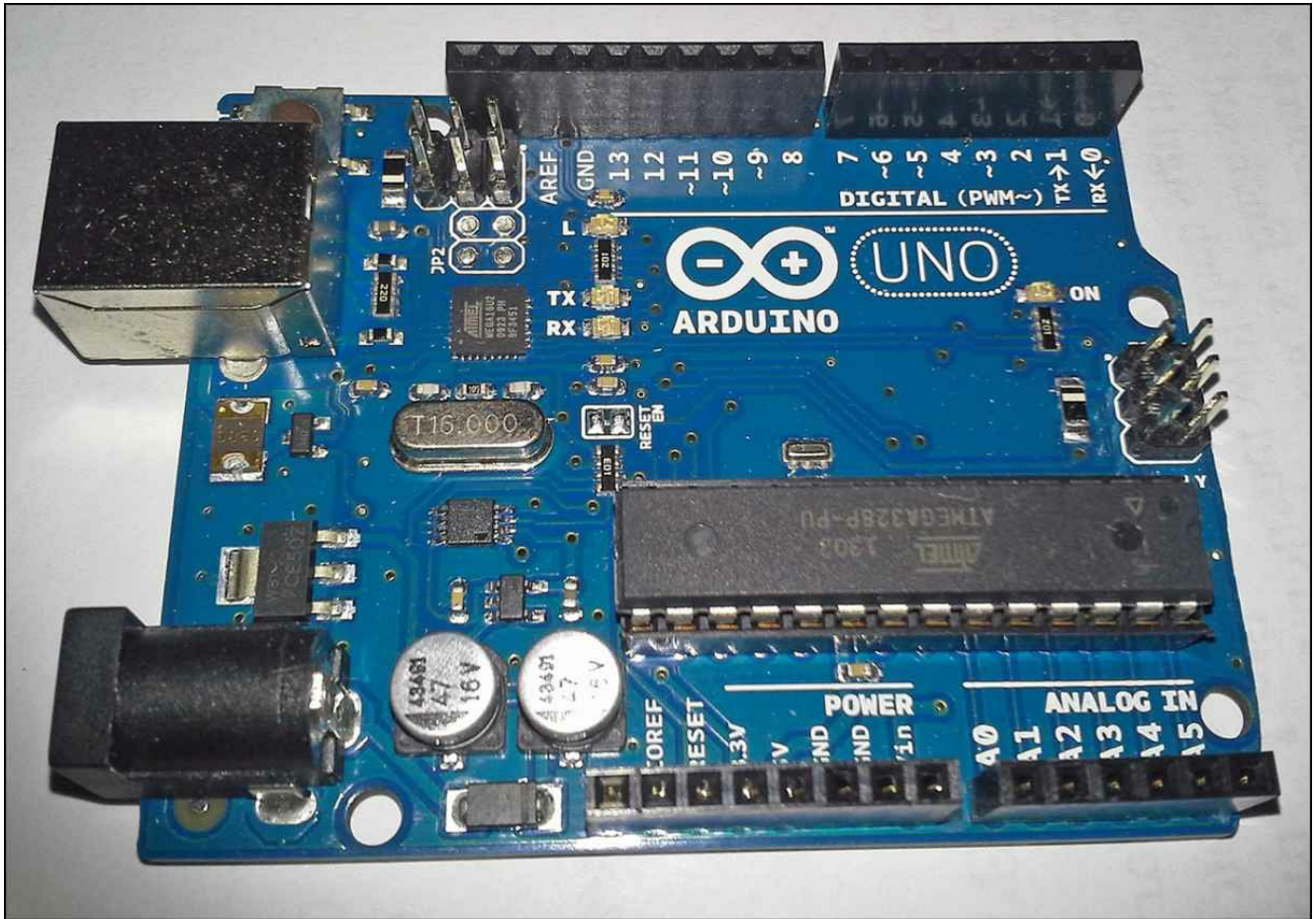
FIGURE 4.5 The Arduino Uno upper and lower header sockets. The lower header socket has 13 ports on it, as described in Table 4.1 .
