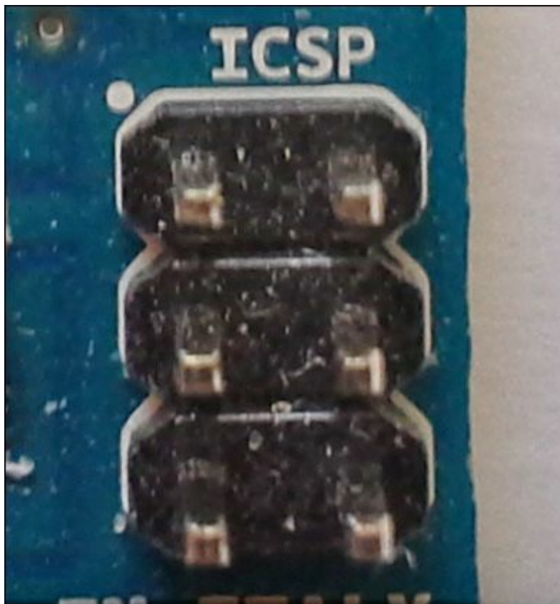
FIGURE 17.2 The ICSP header on the Arduino Uno unit.
